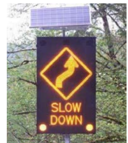
RD11: Example of a dynamic speed feedback sign (Source: ODOT Crash Reduction Factor Manual)
