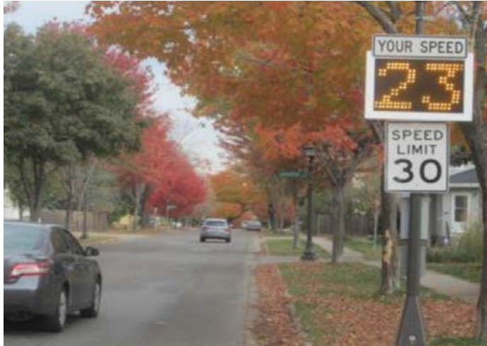
RD12: Example of speed feedback sign (Source: ODOT Crash Reduction Factors Manual)
