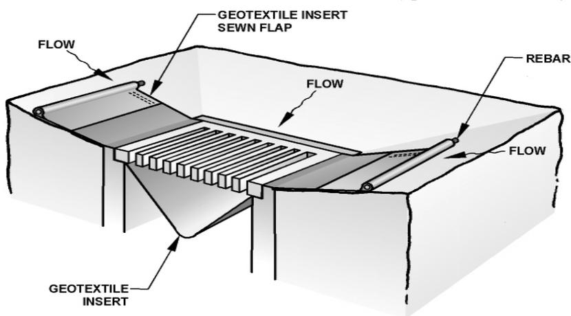
Figure 3-31 Inlet Protection – Geotextile Filter Fabric Insert (Type 3)
