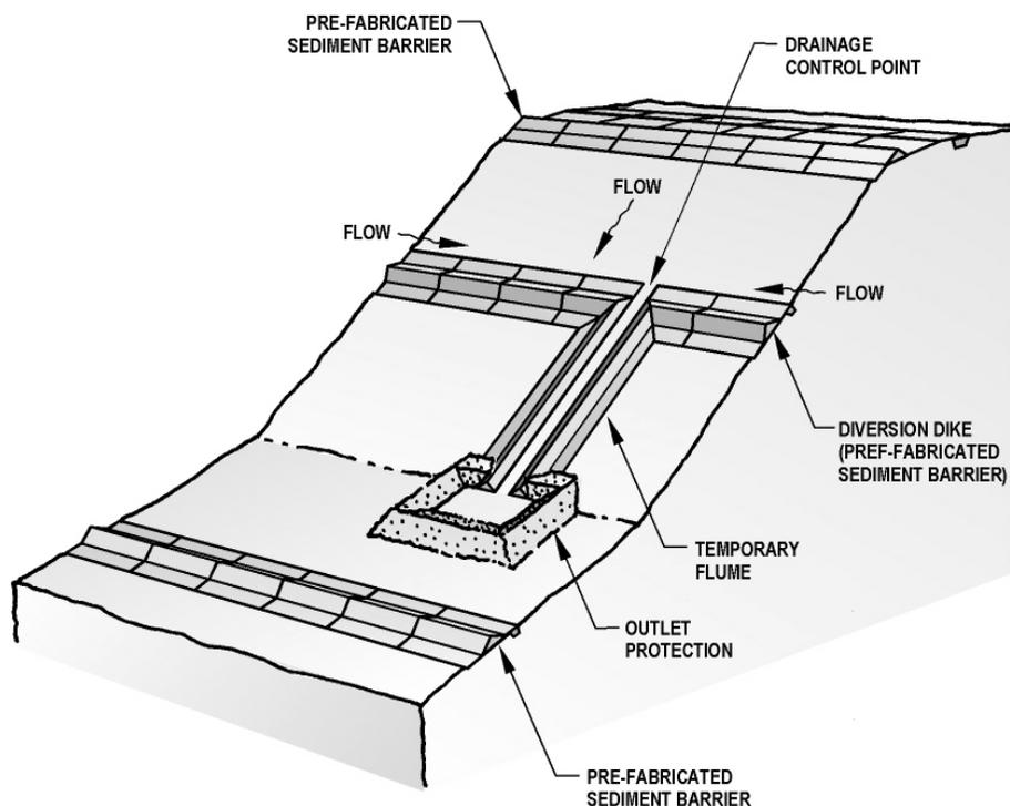
Figure 3-26 Pre-fabricated Barrier System – Sediment Barrier Type 7
