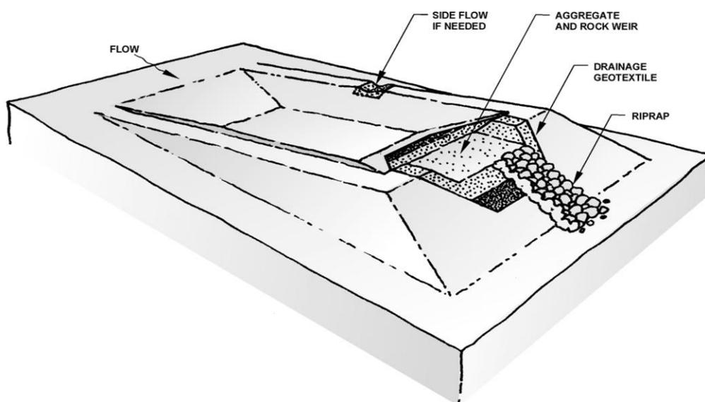
**Figure 3-34 Sediment Trap**
