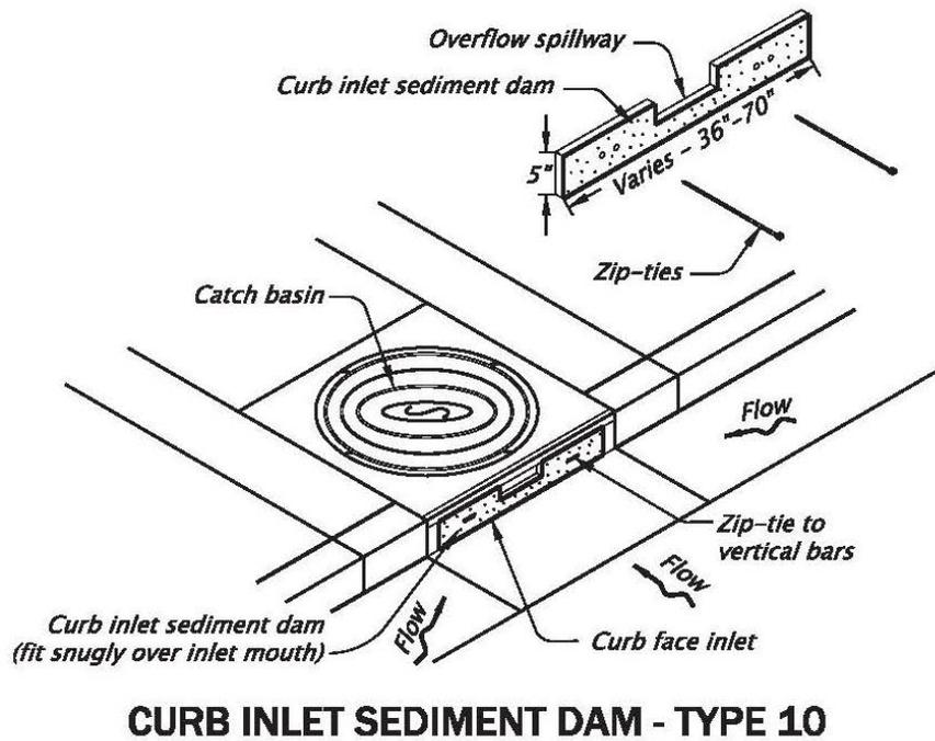
Figure 3-33 Inlet Protection – Curb Inlet Sediment Dam (Type 10)
