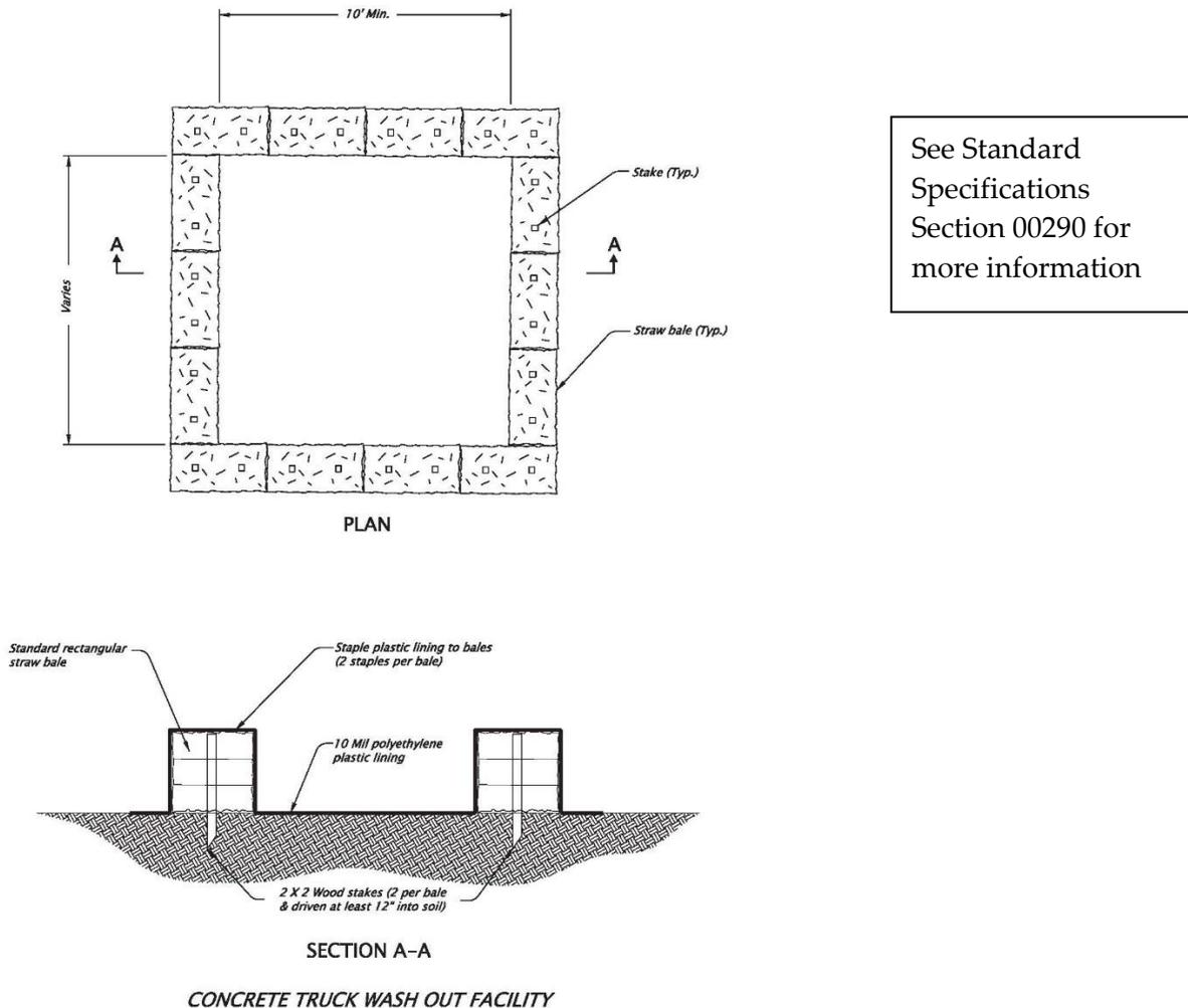
**Figure 4-2 Concrete Washout - Standard Drawing RD01070**
