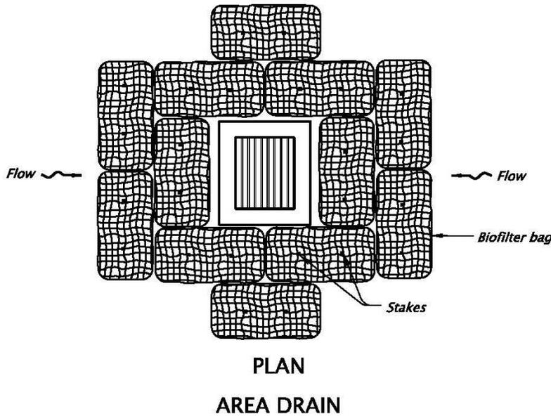
Figure 3-32 Inlet Protection – Biofilter Bags (Type 4)
